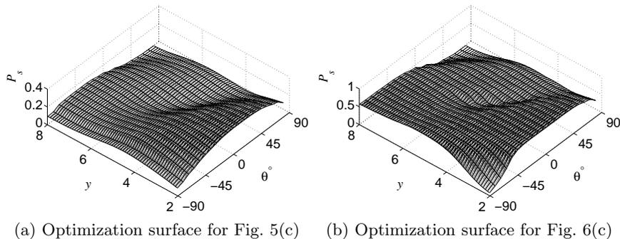
**Fig. 7.** The optimal needle insertion location  $y$ , angle  $\theta$ , and bevel direction  $b$  are found by scanning the DP look-up table for the feasible start state with maximal  $P_s$ . Here we plot optimization surfaces for  $b = 0$ . The low regions correspond to states from which the needle has high probability of colliding with an obstacle or exiting the workspace, and the high regions correspond to better start states.
