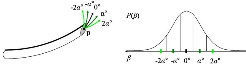
**Fig. 4.** When the needle is inserted, the insertion angle  $\theta$  may be deflected by some angle  $\beta$ . We model the probability distribution of  $\beta$  using a normal distribution with mean 0 and standard deviation  $\sigma_i$  for insertion or  $\sigma_r$  for direction change. For a discrete sample of deflections ( $\beta = \{-2\alpha, -\alpha, 0, \alpha, 2\alpha\}$ ), we obtain the probability of each deflection by integrating the corresponding area under the normal curve.
