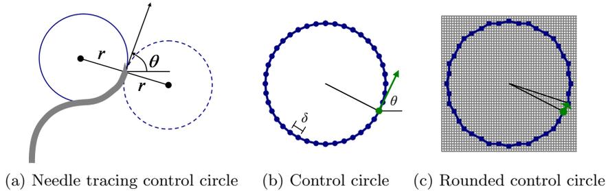
**Fig. 3.** A needle in the bevel-left direction with orientation  $\theta$  is tracing the solid control circle with radius  $r$  (a). A direction change would result in tracing the dotted circle. The control circle is divided into  $N_c = 40$  discrete arcs of length  $\delta$  (b). The control circle points are rounded to the nearest point on the  $\Delta$ -density grid, and transitions for insertion of distance  $\delta$  are defined by the vectors between rounded control circle points (c).
