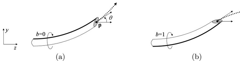
**Fig. 2.** The state of a steerable needle during insertion is characterized by tip position  $\mathbf{p}$ , tip orientation angle  $\theta$ , and bevel direction  $b$  (a). Rotating the needle about its base changes the bevel direction but does not affect needle position (b). The needle will cut soft tissue along an arc (dotted vector) based on bevel direction.
