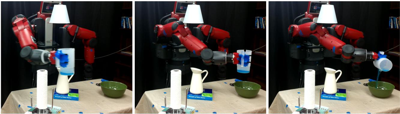
Fig. 6. Baxter robot performing the liquid pouring task with the pitcher (being used as a tool) with blue liquid and the green bowl. The lamp, vase, and paper towel obstacles are white.
