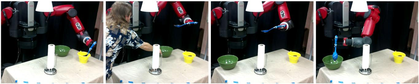
Fig. 4. The Baxter robot performing the powder transfer task with the spoon being used as a tool in blue, the source container in yellow, and the destination container in green. Both the lamp and paper towel obstacles are white.
