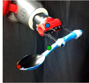
Fig. 5. A spoon being used as a tool in the powder transfer task with an arbitrary landmark at the robot’s gripper marked in blue, the hand-picked landmark at the tip marked in red, and the tool virtual landmark learned by our method marked in green.
