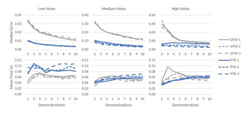
Fig. 7. Results for the simulated drawing task with Gaussian observation noise. PTR exhibited lower error relative to DTW, particularly when only a small number of demonstrations are available.
