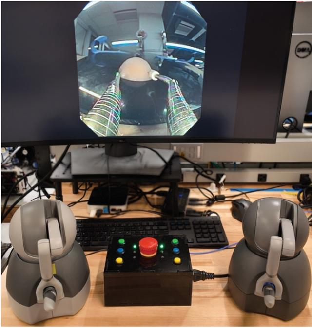
Fig. 7. Example setup of a surgeon control interface for bimanual operation of the endoscopic system
