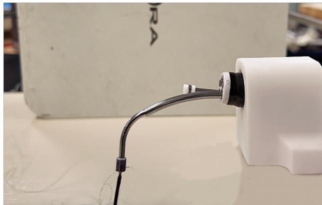
Fig. 6. Experimental setup for workspace validation. Both arms were swept between the joint limits while outfitted with a magnetic tracker on the tip.
