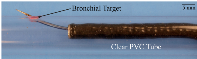
Fig. 4: The concentric tube robot coupled with the tendon-actuated bronchoscope provide flexibility in selecting the position and orientation of the bronchial wall opening. This added dexterity also assists with orienting the initial pose of the steerable needle. Here, the bronchoscope and concentric tube robot are deployed in a clear PVC tube to a desired bronchial target on the wall of the tube.
